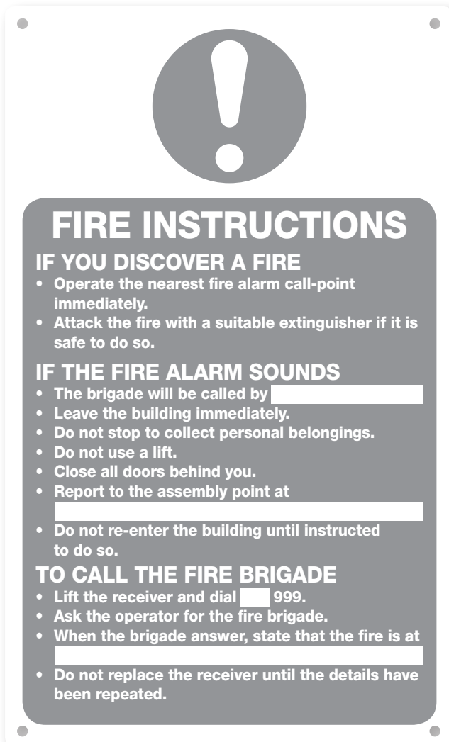
Figure 1: Typical fire action notice
