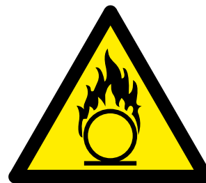
Figure 3 Warning symbol for oxidising agents
