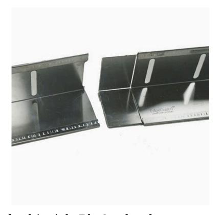
Upon reaching the centre of each 'run', the EdgeGuard can be cut to length using an angle-grinder, hacksaw etc. Extra straight/corner connectors are available for runs of less than 1.2m.
