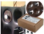
Steel fixing studs and mounting knobs are used for the efficient installation of dimpled sheets, fastening them to concrete and masonry. The mounting knobs prevent the dimpled sheets from tearing the membrane and help to seal the fixing hole.
