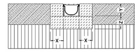
Mark out a trench that is wide enough for your channel drain and at least 100mm of concrete backfill on each side to hold it firmly in place (see illustration, X/Z values). Prepare the base. The channel drain should be assembled after connecting the two half-circle pieces and fixing them to the bottom of the channel drain with four screws. To connect the outlet to a main drain or tooksway, the bottom of the channel can be pieced with a hammer at the pre-marked sections. Last
